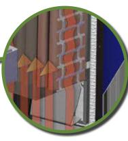
Turbulators in the heat exchanger cause turbulence of the exhaust gas flow through the exchanger. This forces the heated exhaust to better contact the heat exchanger and transfer more of its energy to the surrounding water jacket before exiting out the chimney.
